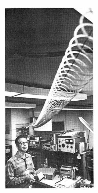
GENE HANSEN (1733) is a Slinky sort. He's found that two of them make a continuously loaded dipole antenna. It's very portable, easily tunable, fairly efficient, and cheap.
